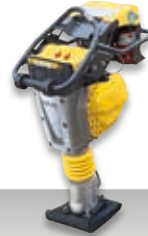
BT 60 G Operating weight: 65 kg Centrifugal force: 15 kN Working width: 230 mm available in DE
